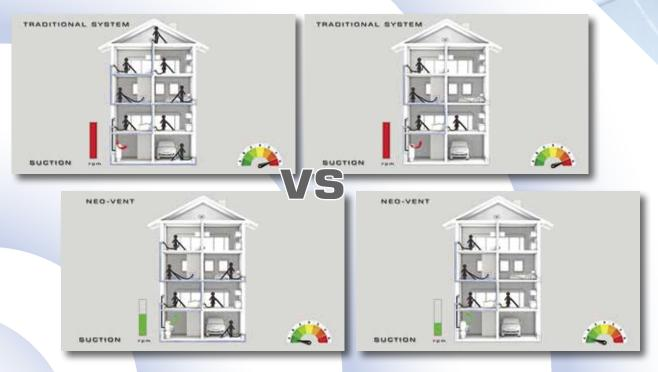
with **NEO-VENT** the speed reduces according to the used air, and the consumed power decreases exponentially according to the speed reduction
