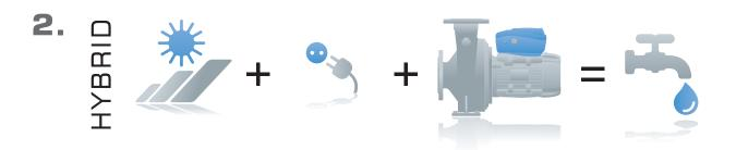
It is possible to connect the pump at the same time to solar panels and to the net or a generator, to make it work when the sun is not enough or during the night.
