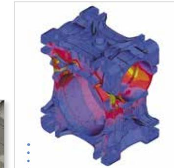
The housing has been designed with parametric three-dimensional CAD SW supported by programs of analysis of the thermal dissipation capacity and the structural resistance/deformation under the effect of working loads.
