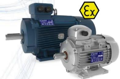
Motive delphi Ex motors differ from standard delphi motors because they are designed to be used, like motive "Ex" gearboxes, in the ATEX zones 1, 2, 21 and 22. Motive delphi Ex motors are in fact certified for such zones according to the norms EN 60079-0 - EN 60079-7 - EN 60079-31 by a notified body.
