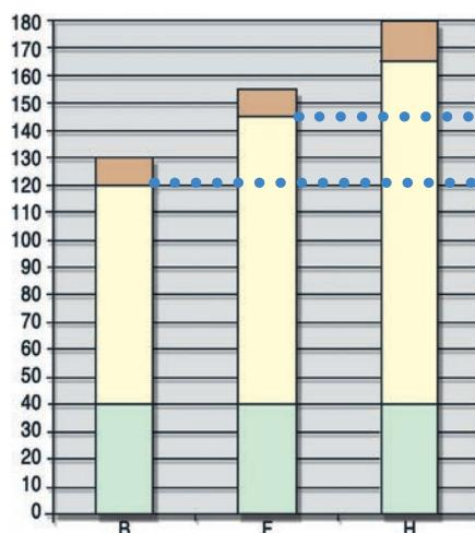
This extra margin gives the motor a "life bonus". As a rule of thumb, insulation life will be doubled for each 10 degrees of unused insulation temperature capability.
