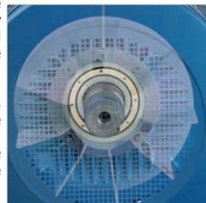
Its purpose is to open the electric circuit between the rotor and the motor frame, thus preventing that the shaft currents go through the bearings and damage their balls surface and roll tracks.
