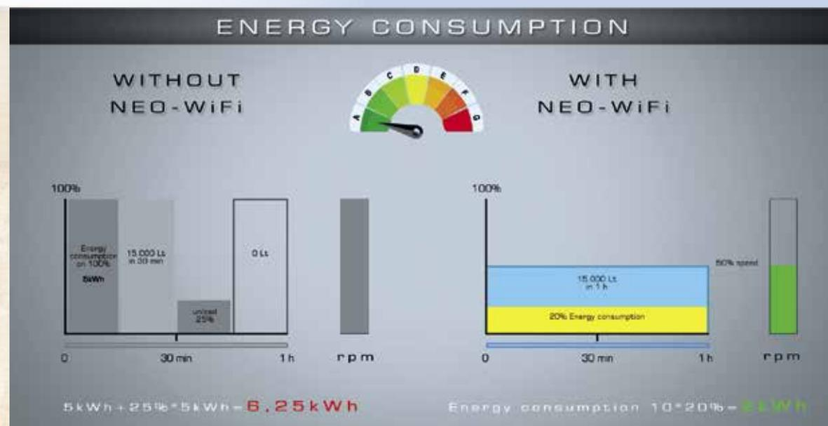
$$\frac{kW1}{kW2} = \frac{rpm1^3}{rpm2^3}$$
