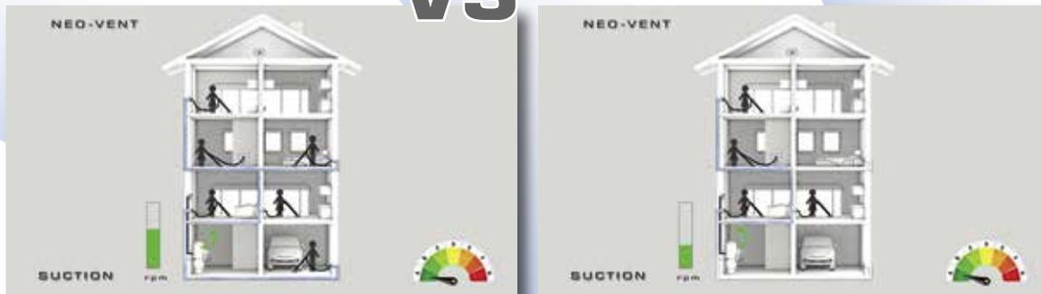
With **NEO-VENT** the speed reduces according to the used air, and the consumed power decreases exponentially according to the speed reduction
