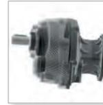
Use of high strength steels and case hardening to  $58 \pm 2$  HRC reduce the wear rate in wheels. All wheels are profile ground to Din 3962 class 6 accuracy for lower noise, higher efficiency and optimized backlash.
