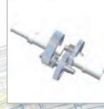
Single stages ratios between 2 and 6, together with proper gears sizes, result mathematically in higher teeth number and size (module) of each wheel and a better fractioned load among the reduction stages. That influences both durability and torque transmission capability.
