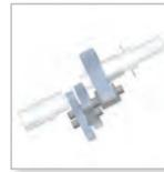
Use of high strength steels and case hardening to  $58 \pm 2$  HRC reduce the wear rate in wheels.
