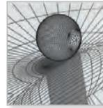
The surface is exposed to a bombardment of micro-spheres that induces compression and increases further the fatigue resistance.
