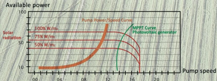
The MPPT is not an operating area for the motor and the use of this power extraction system could unnecessarily limit the delivery of current or voltage to the motor.
