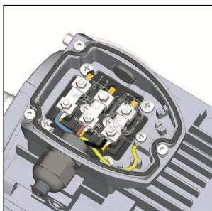
Delta connection is obtained by connecting the end of a phase with the beginning of the following one.
