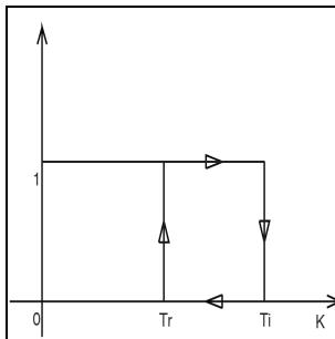
$T_r$ = Opening temperature (motor stops)
