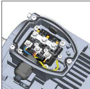
Star connection is obtained by connecting together the terminals W2, U2, V2 and supplying the terminals U1, V1, W1.
