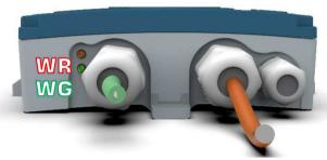
WR: when this red light is on, we have an anomaly (for example, the ethernet cable is disconnected of the network is absent)
