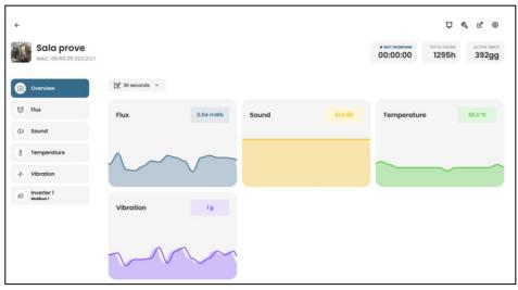
\*NOTE: DOCTOR 4.0's "log rate" (frequency of sending data to the portal) remains anyway still set to one sending per second (this is also why it can be "intelligent"), and it cannot be changed.
