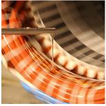
Gel Coat: the stator is then further protected by an epoxy compound which cures fast under hot conditions. Epoxy has very good fungus
